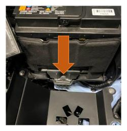
4. Undo the 10mm that connects the induction shield to the battery tray, and the 10mm holding the wiring harness down on the left hand side of the battery tray.
