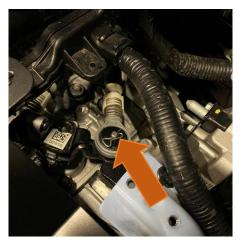
9. Install the supplied mounting post into the quick shift in your desired location, applying the thread lock to the thread before tightening. The furthest hole from the original post hole gives a 35% reduction in shift throw and the closer hole gives 15%.
