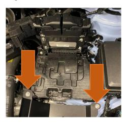
5. Unplug the ECU by pressing the button to release the clamps that then pull up. There are 2 individual plugs on top of the ECU.
