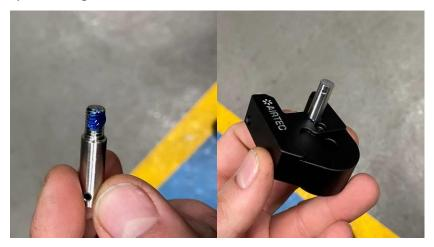
10. Now install the quick shift onto the shifter arm and secure in place using the original R-clip and tighten the grub screw with the thread lock applied into the shifter arm.
