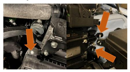
7. Now remove the four 12mm bolts securing the battery tray along with the 10mm bolt holding the wiring loom (highlighted with the blue arrow) on the left side of the battery tray. Remove the tray from the car.
