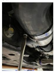
13. Remove the rubber grommet and top hat from the original bracket and insert into your new bracket, attach the bracket loosely to your new larger pipe using the supplied M6 x 12mm hex head bolt and washer.
