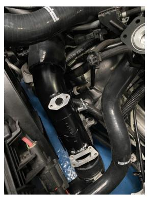
19. You can now build back up the cold side pipe by attaching the MAP sensor to the pipe using the supplied M5 X 12mm with washers, reconnect the plug, attach the solenoid to the mount reusing the original bolt and attach the vacuum line to the take off and secure with the original clip.
