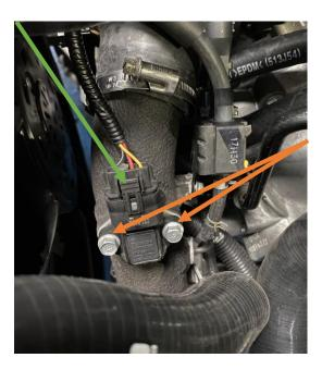
7. Remove the vac line from the takeoff on the pipe by squeezing the clip together and then pulling the hose off and then undo the 10mm bolt holding the solenoid to the pipe.
