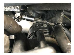
3. Unclip the 2 breather hoses on top of the induction pipe at the back of the engine bay and also the clamp holding on the hose at the front on the induction pipe by squeezing the clips with a pair of pliers and pull the clamp down the hose. The hoses can then be removed by pulling the hoses off the original pipe.
