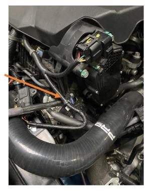
9. From the top you should be able to get access to the hose clip holding the lower silicone to the intercooler, loosen this and then the whole assembly can be pulled out from the car. If you cannot undo this clip from above then undo it after removing the undertray in the following step.
