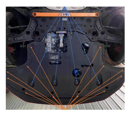
11. Working on the hotside now, undo the 10mm bolt holding on the original pipe to the underside of the engine.
