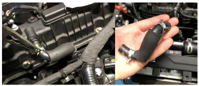
4. Using the 10mm socket undo the unclip holding on the original coolant hose and remove.
