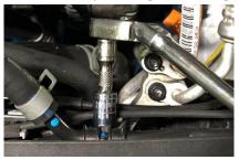
5. Using pliers again squeeze the clip to release it and pull it back so you can release the hose from the coolant tank and also from the T-piece along the front of the engine bay. Taking care as you remove this hose as there may be coolant in the line. You will have to pull the hose out from retaining clip along the back of the plastic panel. Remove the hose from the engine bay.
