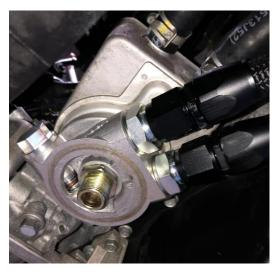
15. Use bracket to clip oil lines to gearbox by loosening the 10mm bolt enough that the bracket can fit between the gearbox housing and the bolt. Once happy with position tighten. Use the supplied oil line separator to attach the oil lines to the bracket with the supplied bolt.
