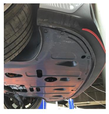
3. In both wheel arches there are 3 plastic clips that need to be removed using a trim tool and then an 8mm bolt.
