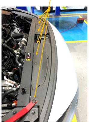
5. The edges of the bumper are now pulled out, best achieved by pulling from the top corner where the bumper meets the front wing and working your way forward with it as it pops out. This is best done with another person doing the other side so that once both sides are pulled forward one person can support the bumper whilst the other disconnects the 3 connectors, 2 on the near side and the other on the off side. The bumper can now come away from the car completely and put aside safely.
