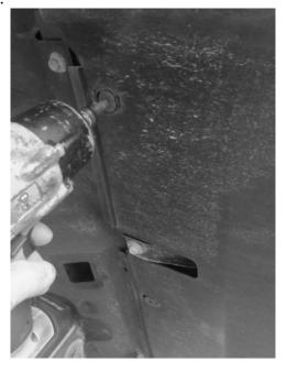
**2**Remove the Phillips Screws on each side of the inner arch liner and two Torx Screws securing the bumper to the wing.
