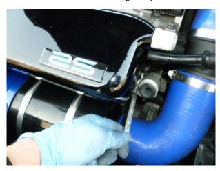
9. Reconnect the hose pictured using the supplied jubilee clip, also reinstall the vacuum pipe using the cable tie provided to secure and finally reconnect the brake vacuum pipe, ensure that it is fully seated. (If you have an RS ECU holder then push this back into place.)
