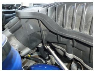
5. Lift the manifold up enough to gain access to the throttle body plug and vacuum hose. Remove these. The inlet manifold can then be removed.
