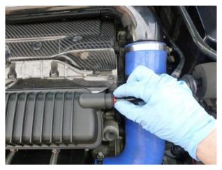
3. If you have an RS Ecu holder fitted you will need to pull this upwards to gain access to the 6 x 8mm bolts securing the inlet manifold. These can be difficult so take your time when undoing these.
