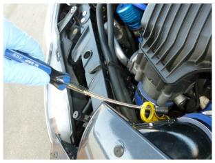
2. Remove the brake vacuum pipe by pushing in the red insert as you pull the pipe outwards.
