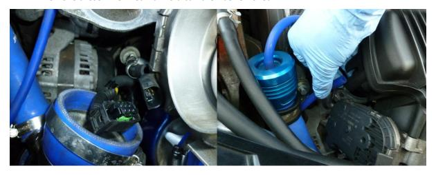
6. Remove the throttle body by undoing the 4 x T30 torx bolts, remove the gaskets from the original inlet manifold and install them along with the throttle body onto your new AIRTEC Motorsports inlet manifold.
