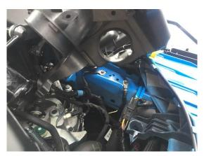
2. Unclip gear selector cable from the standard selector arm.
