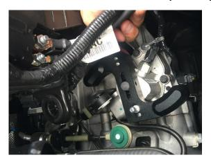
6. Tap fixing dowel in place and clip on selector cable.
