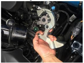
5. Slide new quick shift on the selector shaft and like up locating hole.
