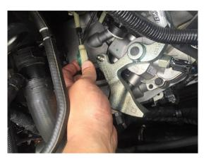
3. With the supplied drift, tap out the fixing dowel on standard selector arm.
