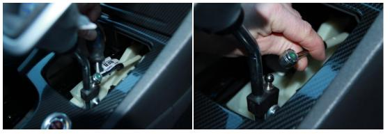
3. Install the 2 piece cable mount onto the lever as low as it will go & then fully tighten the Large Allen keys bolts, then the 2 small bolts
