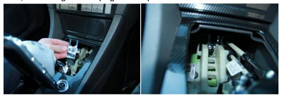
6. Clip cable back in as reverse of removal and then clip end of the cable onto ball end, make sure you have tightened everything before replacing the gear lever surround
