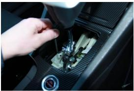
4. Un-clip the cable from the securing mount as shown, you need to push the spring tensioned white part of the clip backwards to release.
