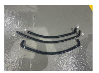
12. Fit hose numbered 1 onto the oil housing then fit 2 onto the bottom of the oil separator.
