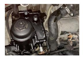
8. Clean surfaces of block then refit new housing in reverse of removal. You can now reconnect the (1) breather hose using the jubilee clip provided.
