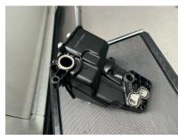
7. Take your old filter top and install new filter provided install new 'O' rings as shown to new housing.
