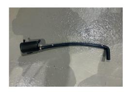
9. Install long breather pipe to bottom of oil separator as shown in picture.
