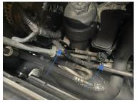
5. Remove 3 x 8mm bolts from front of oil filter housing which secure dipstick tube etc, then remove the 4 x 10mm bolts securing the housing to the engine block, the oil housing can now be removed.
