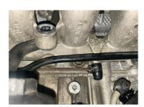
6. Where previously removed (2) discard 90 degree breather hose and install blanking pipe as shown.
