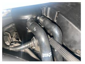
14. For the final hose 5/6 attach as seen in the picture. You can now fit billet hose separator and RS ecu holder or ST Cais.
