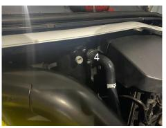
13. Now fit hose 3 onto the oil housing and attach 4 to the oil separator as shown in picture.
