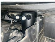
10. Before fitting remove the battery cover, then mark the holes for drilling. (Make sure to check for correct fitment before drilling)
