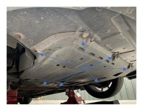
2. Firstly start by removing x7 T30 torques bolts to remove undertray.
