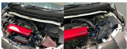
3. Focus ST owners with AS CAIS fitted must lower radiator cradle at this point to remove canister from above. RS owners remove ECU holder by pulling upwards and place to right hand side.
