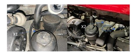
4. Un-plug multi plug from old oil filter housing and secure onto water pipe. This will not be reconnected now remove x2 breather pipes located behind oil filter housing.
