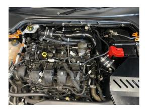
5. Remove the top of the boost pipe where the pipe connects to the turbo.
