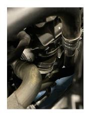
3. You can now start removing the other side by releasing the clip from the intercooler then following the pipe up to the jubilee clip and release it. Then remove the 10mm nut securing the stock boost pipe to the stud on the engine.
