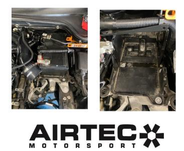
7. You can now access the 2x10mm bolts securing the boost pipe to the engine, once they have been removed you will be able to remove the stock boost pipe.
