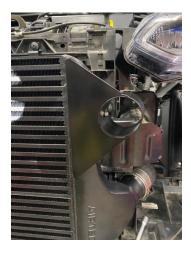
2. You can now attach the air feed hose onto the air feed scoop using the supplied jubilee clip. The air feed can now either go to your AIRTEC Motorsport oil cooler or intake.
