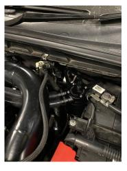
5. Finally, reinstall the engine cover in reverse to Step 1 and ensure routing of the new breather hoses is correct to avoid the cam cover sitting unevenly, as it should sit flat when hoses are routed correctly.
