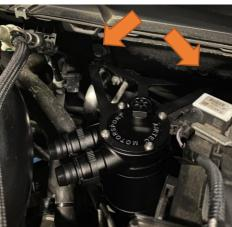
4. Now you can install the silicone hoses. The longer of the two hoses goes to the cam cover and the shorter to the rear intake pipe. Route these under the intake pipe and plumb into the catch can push fit connectors. Use the supplied jubilee clips to secure these onto the cam cover and intake pipe once happy with position.
