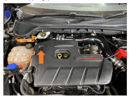
2. Locate the breather pipe connected to the intake pipe and press the blue part of the clip and pull to release it. Do the same the other end of the pipe and remove it from the car.
