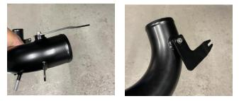
8. Install the silicone reducer onto the turbo elbow and tighten securely. Now install the AIRTEC Motorsport induction pipe by fitting it into the silicone pipe with a supplied jubilee clip. You can then re-clip the breather hose to the lower pipework and reinstall the 10mm bolt to secure it onto the original mounting point.
