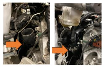
9. You can now align the bracket to the threaded stud on the new induction pipe and reinstall with the original 10mm nut. Reconnect the two breather hose connections removed in Step 5 to the pipework and reinstall the silicone pipework.
