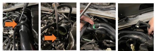
6. Now remove the 10mm bolt from the lower left-hand side of the pipework. After removal, release the lower breather hose by pulling the white clip back. Then you can loosen the jubilee clip located at the bottom to remove the pipework.
