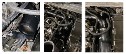
10. Finally, check everything is tight and secure and refit the header tank, engine cover and scuttle panel in reverse of Steps 1 to 4.
