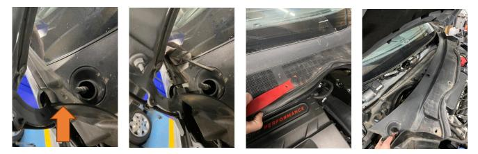
3. Remove the four 10mm bolts from the lower part of the scuttle panel, of which there are two situated in each corner, as shown. Then unclip the pipework attached to the panel above the battery and remove the scuttle panel from the car.
