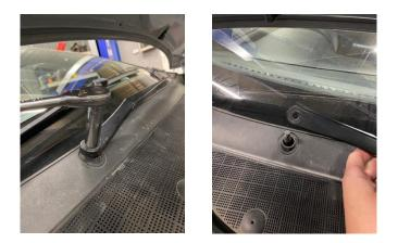
2. Now unclip the rubber edging along the edge of the scuttle panel from where it follows the corners of the windscreen. Once removed, release the five fixing clips positioned across the bottom of the scuttle panel with a trim removal tool.
