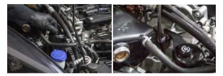
3. Remove original clip on vacuum pipe as shown in attached photo, unclip by simply pulling the blue tab outwards.
