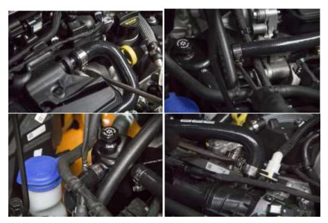
6. Trim engine cover as per guidance below, the breather hoses fail the cover on the underside, it requires some of the foam to be removed to fit the engine cover back on.
