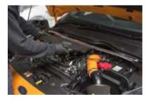
2. Install engine breather onto left hand side of engine as shown in the picture, the breather is secured to the engine with supplied M10 X 16 socket head bolt.
