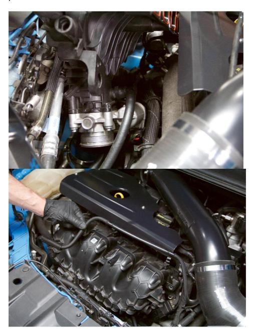
6. Attach the other end of the 90-degree oil breather line fitting to the back of the inlet manifold, using the original clip-on fitting – see picture for reference.
