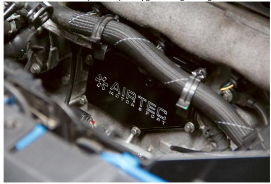
5. Install the straight oil breather line fitting to the AIRTEC Motorsport PCV plate – see pictures for reference.
