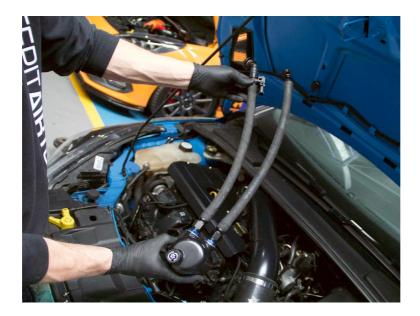
4. Once the oil breather lines are correctly routed and secured in place, the breather tank can be bolted in place to the side of the fuel pump mounting — see photo for reference. Tip, the bracket can be bolted loosely in place, and once the hoses are tightened the bolts can be done up.
