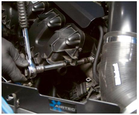
e. Disconnect the throttle body multi-plug by gently pulling the red insert outwards – see picture for reference.
