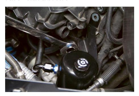
9. Install the breather tank with bracket onto the right-hand side of the inlet manifold – see picture for reference.
