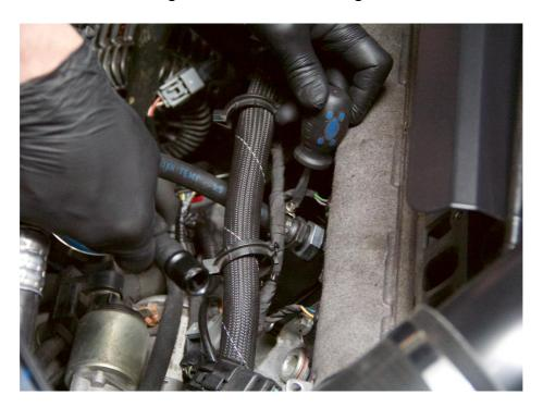
4. Install the AIRTEC Motorsport PCV plate upgrade using the original 8mm bolts.
