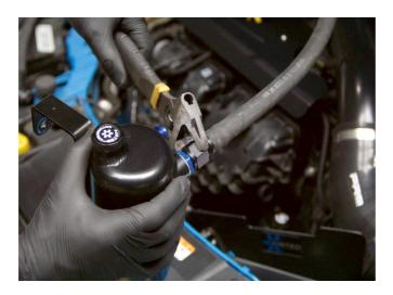
3. Place the oil breather tank in position and route the lines correctly to attach to the top induction pipe and engine cover. Don't forget to re-connect the sensor plug.
