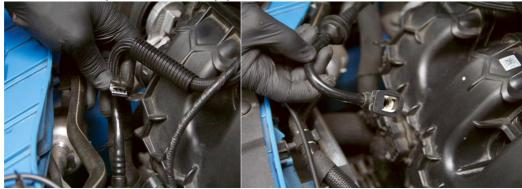
d. Remove the five 10mm bolts that secure the manifold – see both pictures for reference.
