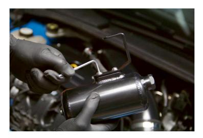
2. Attach the oil breather lines to the tank. The shorter line for the sensor locates on the left-hand side, whilst the longer line locates on the right-hand side.
