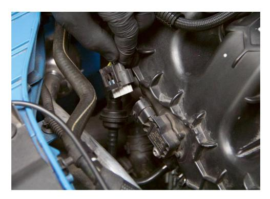
c. Disconnect the push-fit vacuum pipe located on the side of the manifold.
