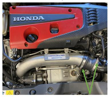
3. Undo the 2 x 8mm bolts and 2 x 10mm bolts holding on the pipework to the original crossover.
