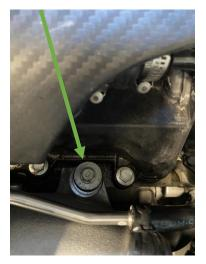
Undo the 2 x 10mm bolt holding the wiring harness on to the side of the crossover.
