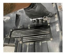
8. Assemble the bracket to the oil cooler as pictured below using the supplied M6 fixings. Note the bracket sits forward of the face of the oil cooler.
