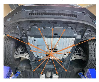
2. Remove the slam panel by firstly removing the 10 x clips holding on the rubber seal at the front and removing before removing the 10 clips holding on the panel itself. It can then be removed.
