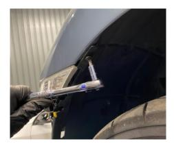
7. With the arch liner removed line up your grill on the arch and mark the holes and around the shape of the grill, from the outside of the grill come in 10mm and draw the shape again. This will be what you will need to cut out. Drill out the holes using a 5mm drill bit and we recommend using a dremel to cut out the shape of the grill. Once cut out then bolt on the grill using the supplied M5 hardware, place the nut on the inside of the wheel arch liner.
