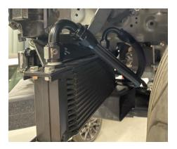
11. Using a suitable container to catch any oil remove the oil filter from the car and then install your thermostatic sandwich plate using the supplied adaptor to tighten. Install the other ends of the oil lines to the sandwich plate and tighten. Before installing wipe a small amount of clean oil around the seal and then before installing a new oil filter again wipe a small amount of clean oil around the seal and then install.
