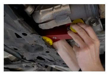
7. Now re install the 17mm and 18mm bolt in reverse of removal and refit the undertray.
