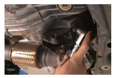
6. Install your new AIRTEC torque mount by rocking the engine forward again then reinstall the bracket when in position.
