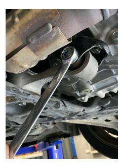
4. You can now remove the mount by rocking the engine forward as this will allow the mount to have enough movement to remove from its location.
