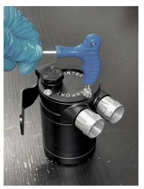
7. Once assembled, the catch can, can now be fitted in its location at the back left of the engine. Use the T40 torx Bit and original bolt to secure the bracket and catch can in place, making sure to line up the second hole with the factory stud on the car.
