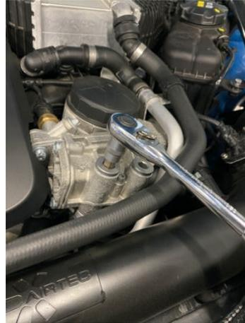
2. Now you can start installing your new AIRTEC billet top covers, make sure to install with provided washer then tighten to 16nm using a torque wrench.
