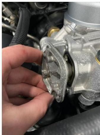
5. Now you can install your new AIRTEC thermostat end cover, secure this in place using a 5mm Allen key with the provided hardware. This is spring loaded so pressure may need to be applied when installing.
