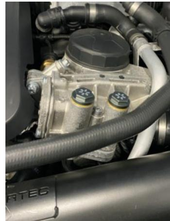
3. Remove engine cover by pulling up from each corner then remove the bolt from the front of the thermostat housing using a E12 socket.
