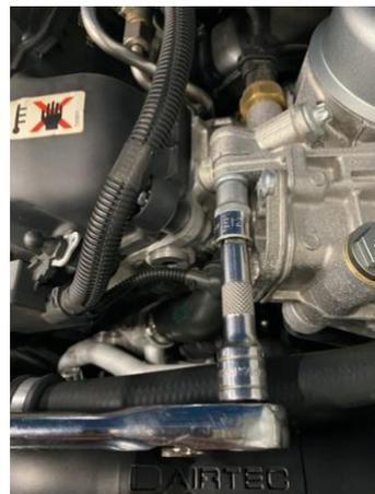
4. You will now be able to access and remove the 2xT30 Torx screws securing the thermostat end cover in place.
