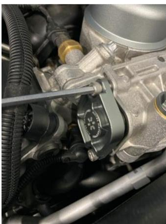
6. Finally reinstall the bolt from the front of the thermostat and check that everything is secured in place correctly.
