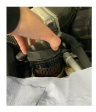
2. After removing the oil filter housing, you can remove the filter and then remove the insert which holds the filter in place. Simply twist the insert then pull it away from the housing.
