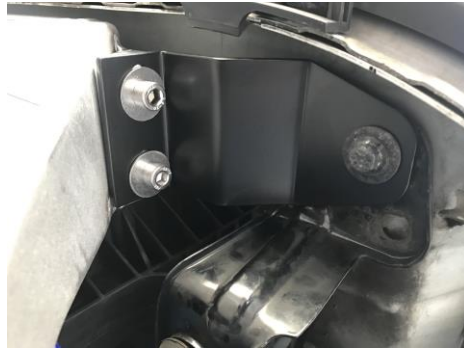
14. Refit boost pipes, check clearances once happy tighten all bolts
