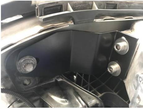
14. Refit boost pipes, check clearances once happy tighten all bolts
