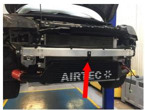
14. Now fit silicon hoses and alloy hard pipes as shown below
