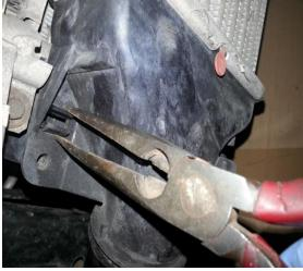
13. Secure the new AIRTEC intercooler pegs into the grommets and mark top fixings against crash bar, remove intercooler and drill marked holes with 7mm drill, re-fit intercooler with bolts provided.
