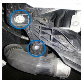
12. Remove 8mm Bolton right of the intercooler + squeeze clip on left side to release , lift intercooler out of pegs
