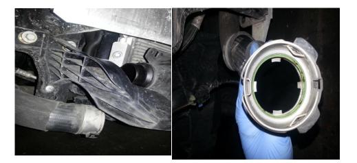
11. Undo the x 2 13mm bolts + drill out rivet holding on the bumper support
