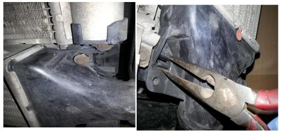
12. Secure the new AIRTEC intercooler pegs into the grommets and mark top fixings against crash bar, remove intercooler and drill marked holes with 7mm drill, re-fit intercooler with bolts provided
