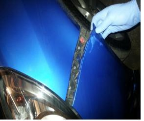
8. Remove air temp sensor plug and remove bumper
