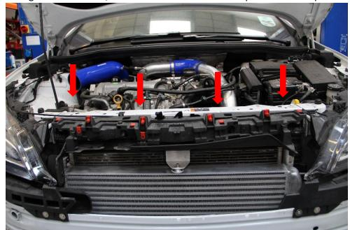
10. Unclip and rotate air guides on both sides of the air con radiator and remove.
