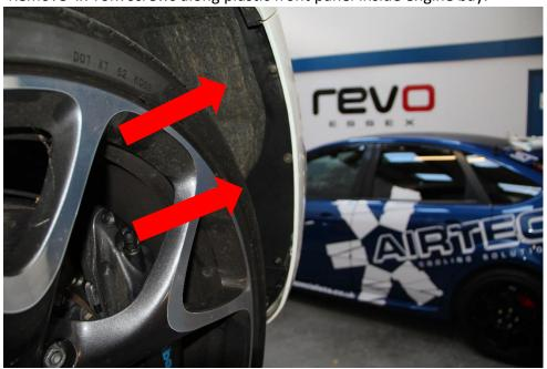
8. Undo bolt and 2 screws to remove air feed for the air box.
