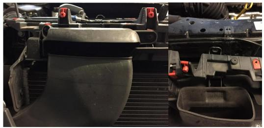
9. Using a 10mm socket, undo the 4 bolts on the front panel and unclip.
