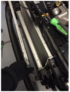
13. Remove both boost pipes using flat blade screw driver to undo C clips where boost pipes connect to the cooler taking care whilst removing air flow sensor from top boost pipe. Pull intercooler upwards and remove.
