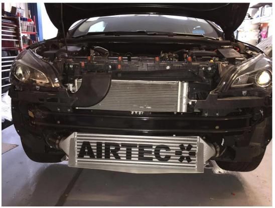
19. Whilst bumper is off, there is a small section of plastic that can be removed from passenger side so all of the AIRTEC cooler can be on show. Remove this and refit
