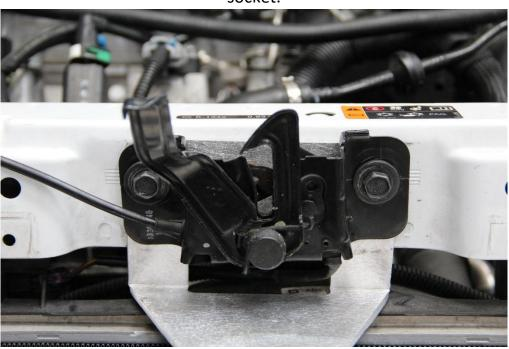
25. Trace the wiring back from the bonnet catch and unplug it. Install the new bonnet catch support bracket, re fit bonnet catch and secure support bracket to intercooler with bolt provided.
