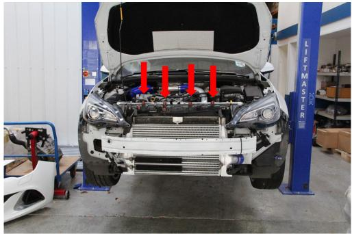
8. Using a 10mm socket, undo the 4x bolts on the front panel and unclip.
