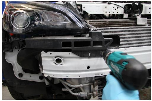
15.Using a 7mm socket undo the 1x screw on the side and 1x screw underneath both head lights.
