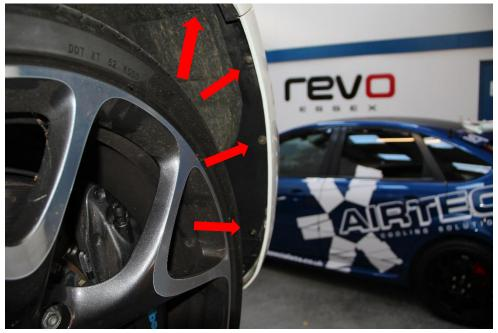
5. Remove 2x E12 Torxs bolts from underneath on both sides of the bumper.
