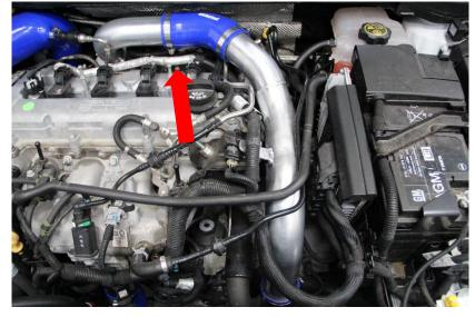
32. Place the alloy link pipe into the end of the silicone hose. This will have to be fed under the coolant pipe work and secure to the original mount with M8 x 20mm Allen cap bolt and Nyloc nut provided. Secure the silicone hose with hose clamp provided.
