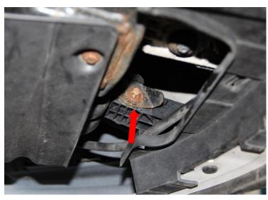
6. Pull the arch liner to one side. Remove the clips on both sides on the bumper inside the wheel arch and carefully remove bumper. Taking caution, unclip the bumper on both sides from underneath the headlight. Carefully pull the bumper away from the vehicle and place away from the vehicle to prevent damage.
