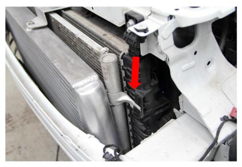
22.Replace the 2x radiator top mounts using a 13mm socket.
