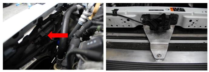
26. Moving to the top of the engine. Remove the engine cover carefully. Using the 7mm hose clamp driver undo both hose clamps. Using an E12 socket to undo the 2x bolts on the standard turbo outlet.
