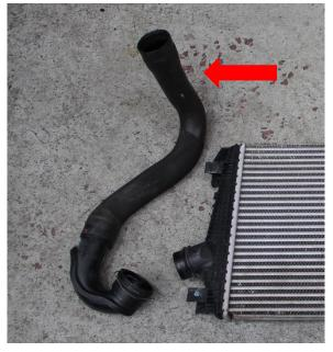
30. Unclip the pipes on the standard boost pipe, using a 13mm socket undo the hard pipe mounting bolt.
