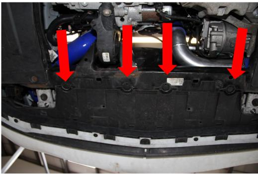
4. Remove 4x T20 Bolts inside both wheel arches, 1x vertical 3x horizontal.
