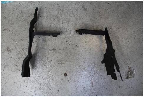
10. Remove the plastic cover from the top of the A/C and intercooler.
