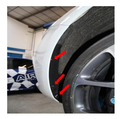
7. Remove 4x T20 Torxs screws along the front panel.
