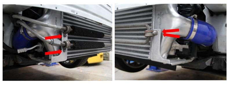
12. Remove the 2x bolts and remove the brackets for the power steering cooler using a 10mm socket.
