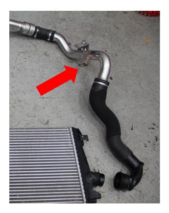
31. Using the 60mm 45 degree silicone hose provided, place the long side on the turbo outlet pipe and secure with hose clamps provided.
