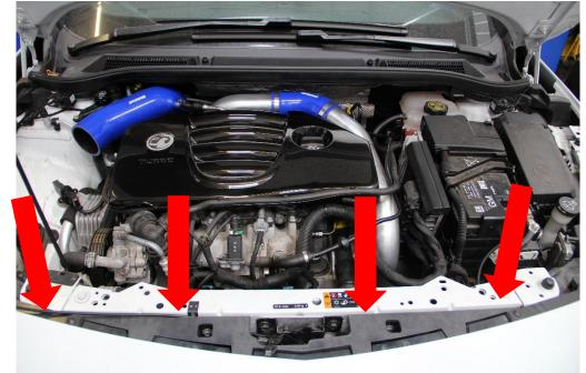
2. Undo and remove 4x T20 Torxs at the top of the bumper.
