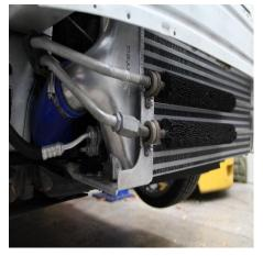
35. Check all hose clamps, fixings are done up and in the correct position. Reassemble your vehicle. Follow the disassembly steps in reverse, you will need to re-rivet the under headlight brace to the crash bar.
