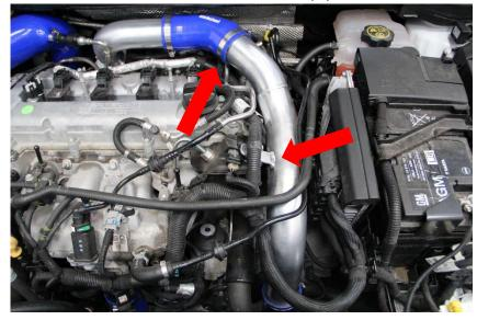
33.Fit the 90 degree silicone hose onto the right hand side alloy pipe, then fit the alloy pipe joiner and install the longer side of the other 90 degree hose to the joiner. The shorter end can now be secured.
