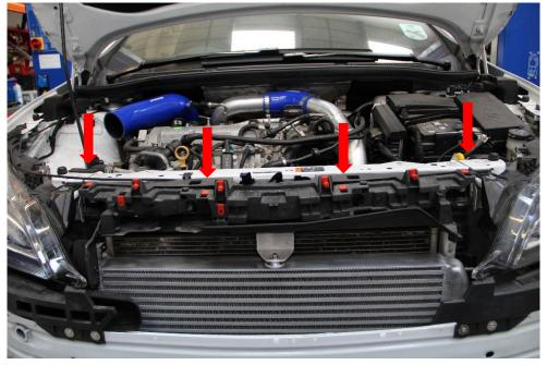
9. Unclip and rotate the air guides on both sides of the A/C radiator using a flat blade screwdriver.
