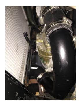
12. Connect straight silicone connector to boost pipe and connect final aluminium boost pipe. Tighten all jubilees and put airflow sensor in the sensor boss on top boost pipe.
