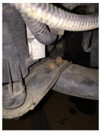
6. Remove aircon radiator bracket. Reattach radiator bracket back into their original positions. (2 torx bolts on each bracket each side of radiator)
