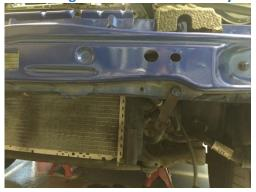
8. Slide intercooler in from below and attach m8 bolts one on each bracket these connect to m8 bosses either side of intercooler. Tighten m8 bolts and nuts holding mounting brackets.
