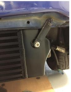
9. Attach steady bracket on top of intercooler 1 m8 bolt on intercooler and 1 m6 bolt and nut in existing bolt hole on crash bar.
