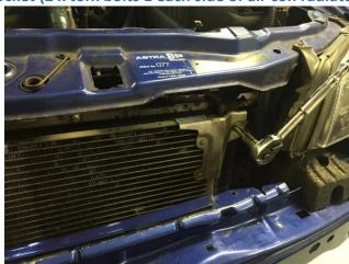
2. Undo aircon pipe work from aircon radiator using a 10mm socket (1 x torx bolt on each connector)
