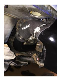
11. Attach straight silicon connector to turbo and tighten jubilee. (If you intend to leave your air con pump attached you will need to trim 20mm of the driver side 45 degree silicone hose) connect aluminium boost pipe from turbo to intercooler and tighten jubilees.
