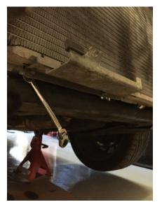
7. Undo 2 x 13mm nuts on crash bar and attach mounting brackets one on each side. Leave bolts finger tight to allow fitting intercooler more easily.
