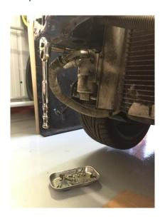
3. remove air con pipe work from air con pump using a 10mm socket (1 x torx bolt on connector)
