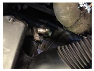
5. Undo radiator bracket using a 10mm socket. Pull the radiator forward about 10 mm
