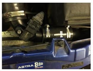
13. Before re attaching bumper trim adjustment brackets on fog lamp units as shown in picture. Check all bolts and jubilees are tight then reattach bumper.
