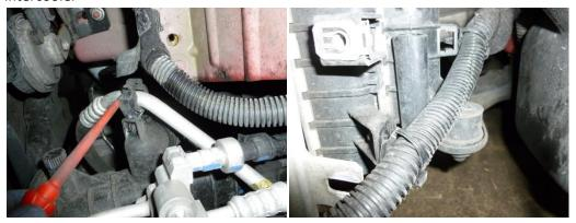
18. Remove 2 x T10 bolts securing top of standard intercooler to radiator, then remove top rubber hose
