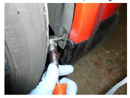
3. Bottom of bumper - remove 3 securing pins by pulling centres of pin out first
