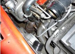
19. Now un-clip intercooler top from radiator and remove both top intercooler pipes
