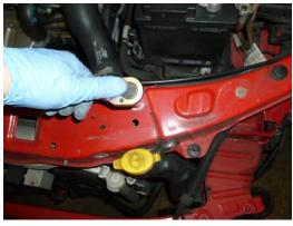
12. To remove slam panel, lift upwards, un-clip Air feed pipe and un-clip wiring loom from panel so it's free to be removed and placed to one side.
