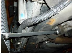
26. Reposition horns on top of each other as shown
