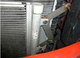
24. With the A/C radiator secured we can fit the Intercooler, place the intercooler as shown and check you have @ least 5-10mm clearance from the original fan assembly
