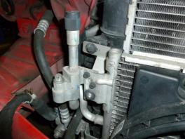
23. With the left hand side secured we can now secure the right hand side. Place the alloy spacer as show and use bolt provide to secure (goes though back of radiator), the bracket will hook into the radiator and secure with original fixings
