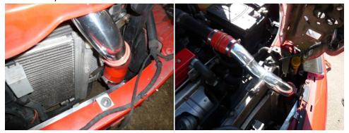
30. With the slam panel fitted check clearance of alloy boost pipe to the panel itself, if required install protective edging supplied, if hitting readjust alloy boost pipe and silicon hoses to give you enough clearance.
