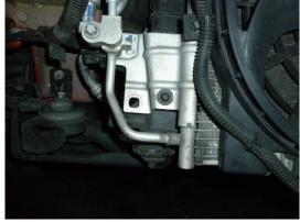
22. Take the small 'L' shaped bracket and place on the standard radiator , use original bolt and tread fixing taken from standard Vauxhall intercooler
