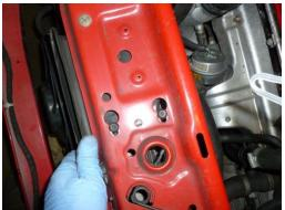
13. Remove the 2 jubilee clips on the left & 1 jubilee clip on the right hand side of the alloy boost pipes
