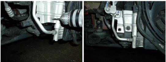
22. Take the small 'L' shaped bracket and place on the standard radiator , use original bolt and tread fixing taken from standard Vauxhall intercooler
