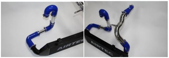
28. On to the right hand side and install the 45 degree silicon hose from the kit onto the intercooler , then install 'S' alloy boost pipe as shown and fit hump hose to alloy pipe onto original Vauxhall boost pipe, then once happy with position tighten hoses and fit securing bolt for Alloy boost hose
