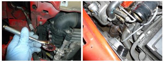
19. Now un-clip intercooler top from radiator and remove both top intercooler pipes
