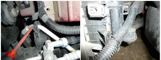
18. Remove 2 x T10 bolts securing top of standard intercooler to radiator, then remove top rubber hose
