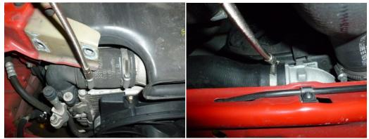
14. Remove Torx10 bolt and remove pipe
