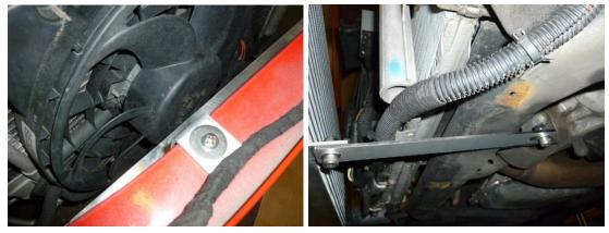
26. Reposition horns on top of each other as shown
