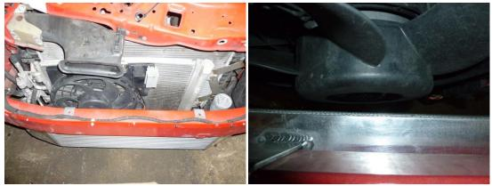
25. Drill 2 x 5mm holes (no bigger) and secure with screws provided (Tip. Use the lower securing brace to help position the intercooler before drilling). Once intercooler is secure install lower brace as shown
