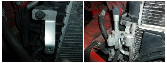
23. With the left hand side secured we can now secure the right hand side. Place the alloy spacer as show and use bolt provide to secure (goes though back of radiator), the bracket will hook into the radiator and secure with original fixings
