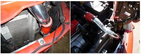
29. With the slam panel fitted check clearance of alloy boost pipe to the panel itself, if required install protective edging supplied, if hitting readjust alloy boost pipe and silicon hoses to give you enough clearance.
