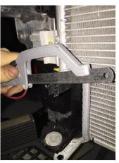
12. Secure the new AIRTEC intercooler pegs into the grommets and mark top fixings against crash bar, remove intercooler and drill marked holes with 8mm drill, re-fit intercooler with bolts provided
