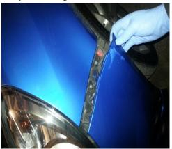
7. Remove air temp sensor plug and remove bumper
