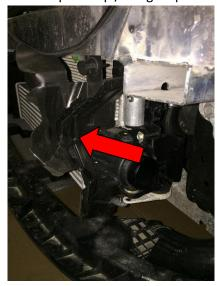
13. Remove 8mm Bolton right of the intercooler + squeeze clip on left side to release, lift intercooler out of pegs.
