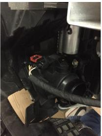
12. Unclip air scoop each side of cooler 1 push clip / 2 tags top and bottom
