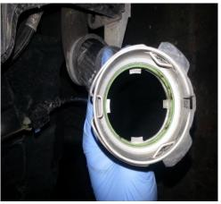
11. Unplug MAF sensor on intercooler and install into new Airtec intercooler.
