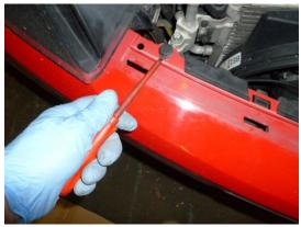
7. Remove foam end caps of crash bar and drill out alloy rivets as shown
