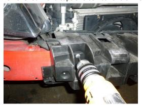
8. Remove 10mm bolt securing washer bottle
