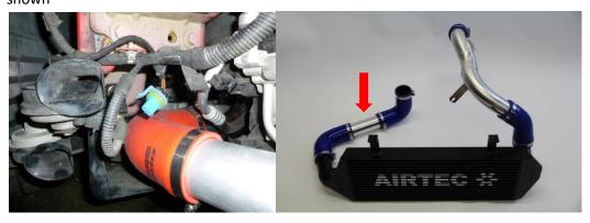
17. On to the right hand side and install the 45 degree silicon hose from the kit onto the intercooler, then install 'S' alloy boost pipe as shown and bolt to original intercooler fixing stud as shown, fit hump hose to throttle body, then once happy with position tighten hoses and fit securing bolt for Alloy boost hose
