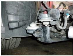
16. Now it's time to install the boost pipes, take the 90 degree reducer (50mm-60mm) and place 50mm end onto the turbo compressor housing, then connect the alloy straight joiner as shown
