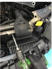
12. Unclip wiring loom from bottom of intercooler and remove intercooler
