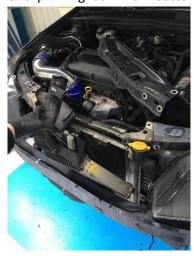
13. With intercooler and pipework removed, it's time to fit your new Airtec intercooler!
