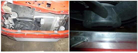
14. Drill 2 x 5mm holes (no bigger) and secure with screws provided (Tip. Use the lower securing brace to help position the intercooler before drilling). Once intercooler is secure install lower brace as shown
