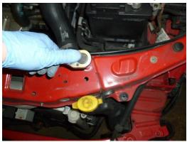
10. To remove slam panel, lift upwards, un-clip Air feed pipe and un-clip wiring loom from panel so it's free to be removed and placed to one side.
