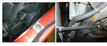
15. Reposition horns on top of each other as shown
