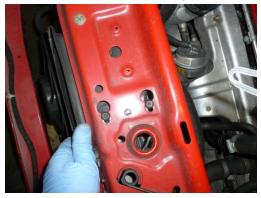
11. Remove standard intercooler by undoing 1x 10mm nut & 1 E8 torx bolt
