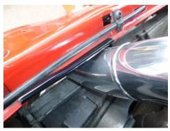
20. All whats left to do now is refit bumper etc in reverse order of removal. Please note trimming needed for bottom of bumper fixing to subframe.
