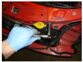
9. Remove the 6 x 13mm bolts securing the slam panel (3 each side)
