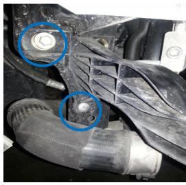
12. Remove 8mm Bolton right of the intercooler + squeeze clip on left side to release , lift intercooler out of pegs
