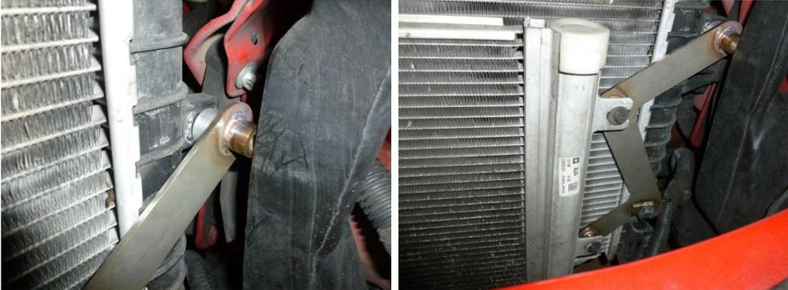
24. With the A/C radiator secured we can fit the Intercooler, place the intercooler as shown and check you have @ least 5-10mm clearance from the original fan assembly
