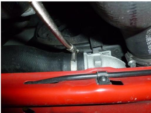
14. Remove Torx10 bolt and remove pipe
