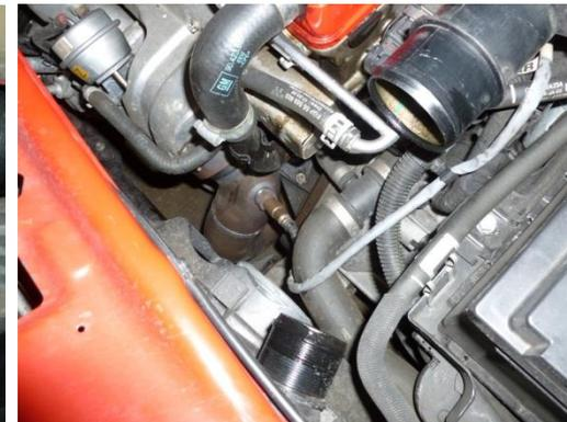
19. Now un-clip intercooler top from radiator and remove both top intercooler pipes
