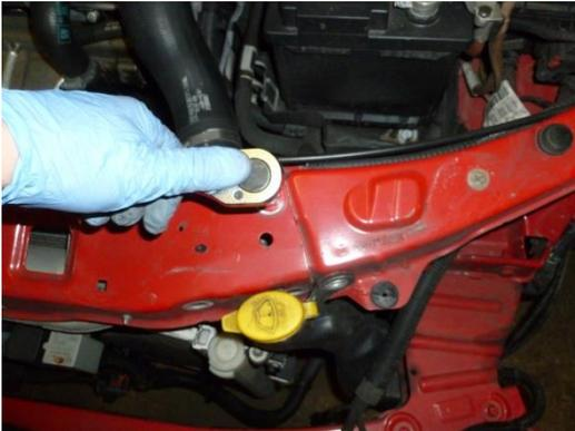
12. To remove slam panel, lift upwards, un-clip Air feed pipe and un-clip wiring loom from panel so it's free to be removed and placed to one side.
