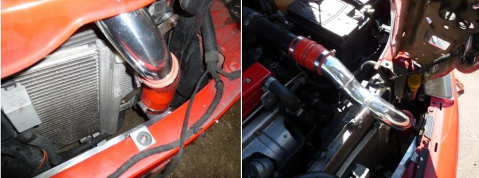
30. With the slam panel fitted check clearance of alloy boost pipe to the panel itself, if required install protective edging supplied, if hitting readjust alloy boost pipe and silicon hoses to give you enough clearance.
