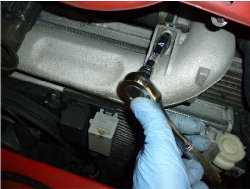
15. Undo the jubilee clip on the Turbo and remove the rubber connecting hose
