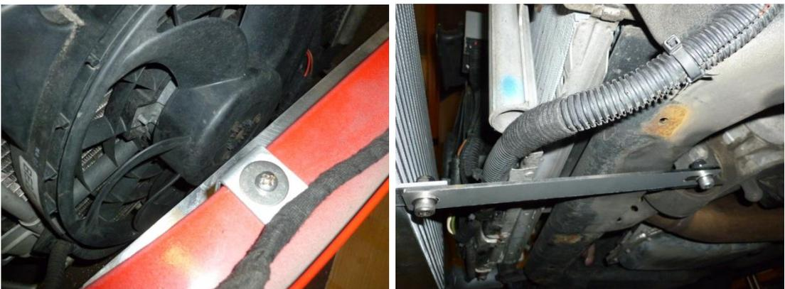
26. Reposition horns on top of each other as shown
