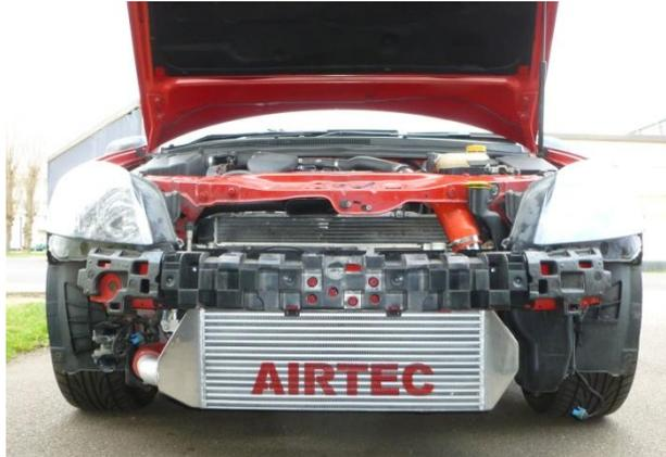
1. Remove front grill (3 x T25 Torx bolts) then pull upwards, be careful not to break clips.
