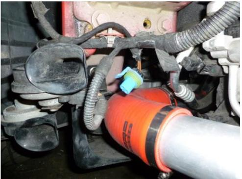
29. On to the right hand side and install the 45 degree silicon hose from the kit onto the intercooler , then install 'S' alloy boost pipe as shown and fit hump hose to alloy pipe onto original Vauxhall boost pipe, then once happy with position tighten hoses and fit securing bolt for Alloy boost hose
