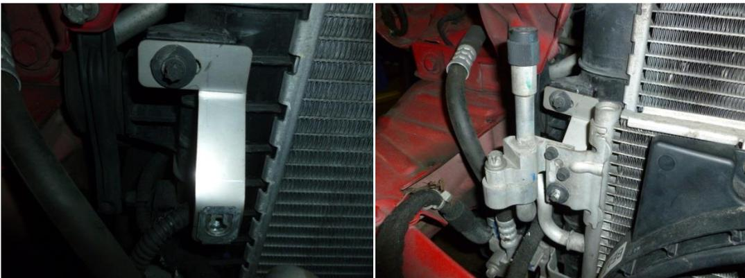
23. With the left hand side secured we can now secure the right hand side. Place the alloy spacer as show and use bolt provide to secure (goes though back of radiator), the bracket will hook into the radiator and secure with original fixings
