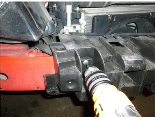
9. Remove headlight bolts (3x 8mm bolts) then un-clip by pulling red centre insert out of clip
