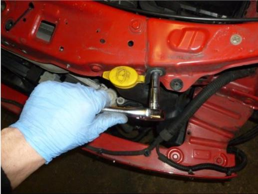
11. Remove the 6 x 13mm bolts securing the slam panel (3 each side)
