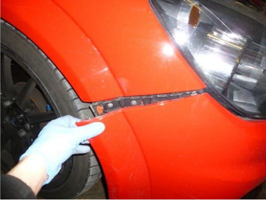
5. Disconnect the fog light wiring 'Blue clips'
