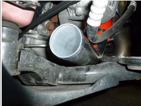
28. Following on from step 27 take the 90 degree silicon hose from the fitting kit and connect intercooler left hand outlet to the alloy pipe fitted in step 27. Take some time getting silicon hoses and alloy pipe in the correct position so it doesn't hit anything, then you can tighten.
