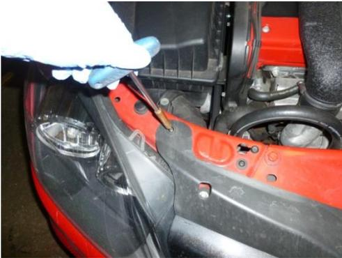
2. Remove the 4 x T20 screws, securing the inner wheel arch liner to the bumper
