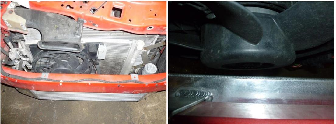
25. Drill 2 x 5mm holes (no bigger) and secure with screws provided (Tip. Use the lower securing brace to help position the intercooler before drilling). Once intercooler is secure install lower brace as shown
