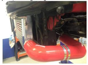
24. Install alloy pipe as shown, this will connect to the 90 degree silicon hose, must also install alloy spacer as shown + map sensor
