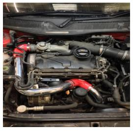
28. FITTING EGR DELETE. Remove old egr and install blanking plate and gasket supplied 'use original bolts' then install egr pipe with new fittings supplied, fit vac pipe take off and old vacuum pipes are now obsolete
