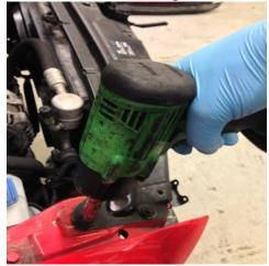
7. Carefully remove the cradle and support the rad pack with a trolley jack
