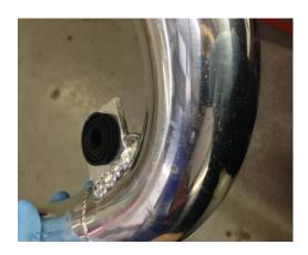
27. NOT FITTING EGR DELETE. With the alloy top pipe fitted, fit the 90 degree silicon hose to standard EGR or a previously fitted egr delete
