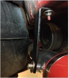
23. PASSENGER SIDE 'UK'. Fit 90 degree silicon bend from intercooler then install alloy joiner, then long 90 degree. Side shield will require cutting or removing
