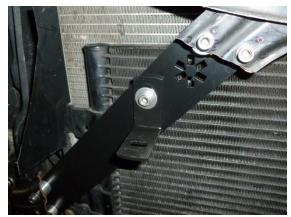
17. Bend 3 x tabs located on the radiator support upwards as shown
