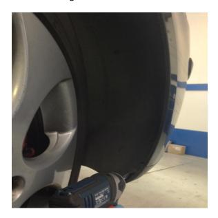
3. Remove the x4 plastic clips holding bumper to radiator cowling, remove fog light surrounds and unclip bumper.
