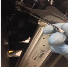
6. Remove standard crash bar x6 13mm bolts and several T27 torx bolts
