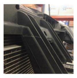
8. Now you need to secure the intercooler brackets, you will need to 4 holes to gain access to the bolts securing the Air-con radiator, these are used to secure the brackets. Note. top left requires extra cutting on Polo Gti 'as shown'.
