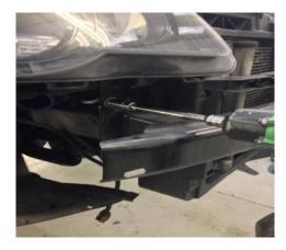
7. Due to the increased size of the Airtec intercooler you will need to cut the top of the crash panel as shown above, use hack-saw, Air saw, dermal or angle grinder with thin cutting disc.
