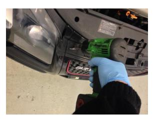
2. Undo x6 T20 torx screws securing inner arch to bumper & x 2 torx screws securing bumper to wing.
