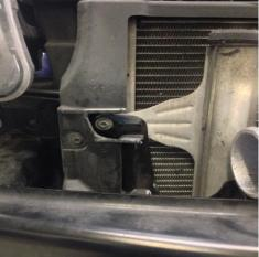
9. Fit intercooler and pipe work as show in photo, both sets of pipe work connect to the original pipes.
