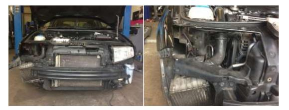
3. Secure new intercooler side brackets, these are located behind the plastic crash panel, an easy way to fit is to drill larger holes then you can gain access to the Aircon securing bolts that you will use to fit the new side bracket. See photo's below
