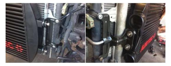
4. Once intercooler is secure fit top boost pipe, take note of pipe layout in the below photo
