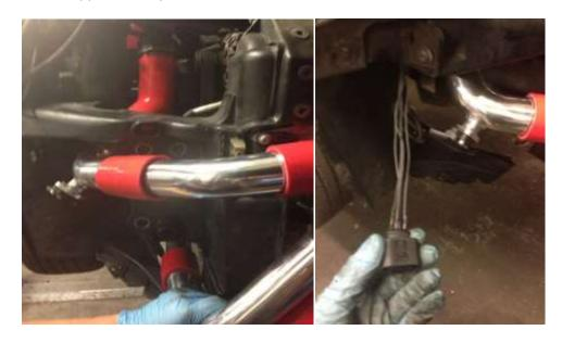
6. The top boost hose connects to the standard OEM plastic boost hose with the Alloy billet connector, please remember to swap the 'o' ring from the standard boost hose and place onto billet connector
