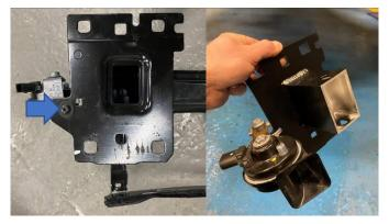
17. Fit the crash bar feet reusing the original bolts removed in Step 13 but do not fully tighten.
