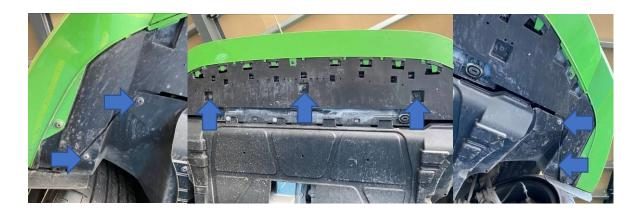
6. Using a second person to help, you can now pull the edges of the bumper to release it. On the passenger side, towards the bottom of the bumper you will see the wiring plug that connects to the front bumper. Disconnect this and then you will need to remove the pipe going to the headlight washers (you will need a suitable container to catch the fluid that comes out). The bumper can then be removed and placed safely aside.
