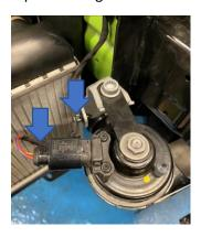
10. Unclip the air temperature sensor by squeezing the clip at the front of the temperature sensor.
