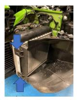
9. Disconnect the horns and unclip the wiring harness from the bracket.
