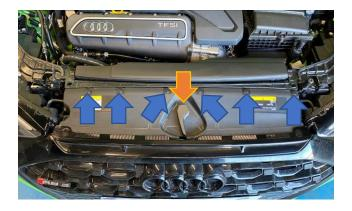
3. Underneath the panel there are two foam parts (orange arrows) that need to be removed by simply pulling them and then remove the three T27 Torx bolts (blue arrows).
