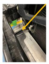
13. Remove the four 16mm bolts and one T27 bolt holding the crash bar to the car. The crash bar then lifts up, tilts forwards and comes off going up through the cut outs in the rad pack.
