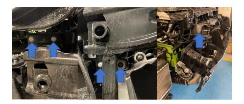
14. Undo the hose clamps going to the original intercooler and then undo the two T30 bolts holding the intercooler. Then lift it up to release from the lower brackets and remove.
