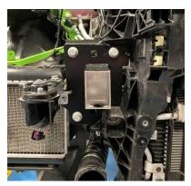
18. Place the intercooler onto the car and use the supplied M12 bolt, washer and nut each side to secure but again **do not fully tighten at this stage**.
