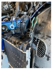
6. Remove the 2xT15 screws from underneath the radiator. You can lift the radiator up and remove it from the car.
