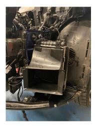
5. The hoses will now need to be removed from the radiator, to do so clamp the hoses so that you wont loose much fluid then using hose clamp plies release the clips and pull the hose off of the radiator. (We recommend having something underneath the hoses to catch the excess fluid)
