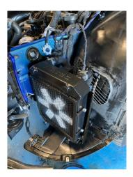
8. Secure the auxiliary radiator in place using the provided 2x10mm hex head bolts with washers. You can now refit the ducting onto the radiator by sliding the slotted mounting points onto the pins.
