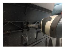
3. Now remove the 3x T30 Torx holding bumper to crash bar and unclip the bumper from the wings. The bumper can now be removed, whilst doing so disconnect the wiring harness and unclip the washer jet hose.
