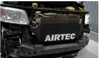
16. Some slight trimming to the front bumper will also need to be made on either side for the intercooler to fit.
