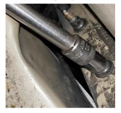
6. Locate the power steering reservoir inside the engine bay and remove 10mm bolt securing reservoir to the front bumper. You can now rest the reservoir in a safe place in the engine bay. Now you can remove x2 T20 torx screws where this was located.
