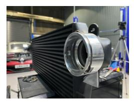
15. Now install your new AIRTEC intercooler by reusing oem fitting points and oem fittings.
