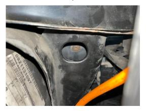
8. Using a trim tool lever out the 3 front bumper mouldings, behind these you will find T27 screws that will need to be removed.
