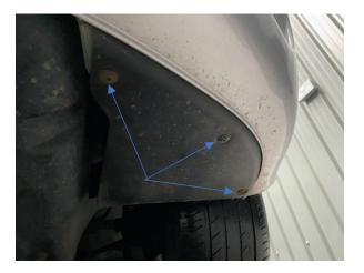
5. Remove x1 T20 torx inside arch and x2 10mm nuts securing bumper to arch.
