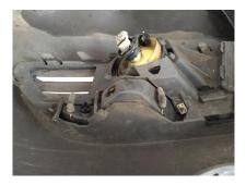
7. Remove poly from slam panel & air guides from rad pack (Remove air sensors from N/S scoop).
