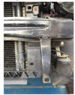
10. Offer up new cooler, mark two points for mounting brackets & drill 6mm whole.
