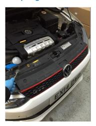
2. Remove 4x T20 screws inner arches.
