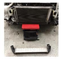
20. Install new intercooler with brackets provided.
