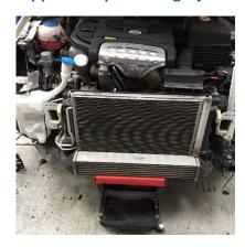
19. Un-clip standard intercooler on the right hand side then un-hook left hand side.
