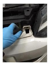
8. Remove head lights and remove 5x T30, 1x T20 then remove top metal supports.
