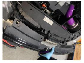
2. Undo 4x T25 Torx holding inner arch to bumper.
