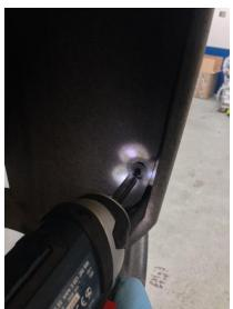
3. Undo 1x T25 Torx holding bumper to arch.
