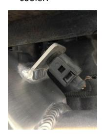
13. Relocate horns with supplied brackets.
