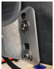
12. Remove temp sensor from original bracket and clip onto cooler.
