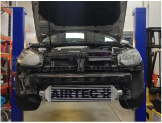
11. Bolt intercooler in place with screws supplied.
