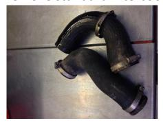
9. Swap 'o' ring from standard boost hose to alloy pipe connector10. Place intercooler in position secure with fixings provided
