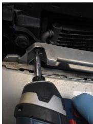
6. Remove bumper making sure to unplug fog lights & headlight washer pipe.
