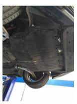
3. Remove 4 screws from wheel arch.
