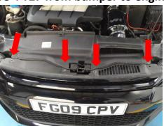
6. Remove bumper and disconnect fog lights & side lights.
