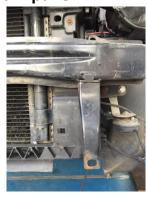
10. Offer up new cooler, mark two points for mounting brackets & drill 6mm whole.
