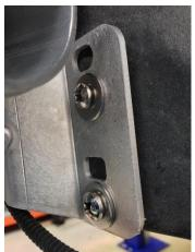
11. Remove temp sensor from original bracket and clip onto cooler.
