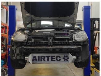
10. Bolt intercooler in place with screws supplied.
