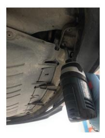
5. Undo 2x T25 Torx securing top of bumper
