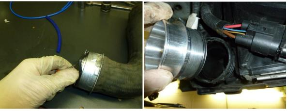
10. Left hand Pipe layout. It may take a couple of attempts to get the hose fitting correctly and some cutting of the hose at the points. Check twice, cut once! You can cut some more off, but you can add it back on as easy.
