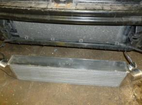
6. Turn Airflow multi as show so it does not fail crash bar, then using the 4 x 10mm self tapping bolts fit to existing bolt holes as shown below.
