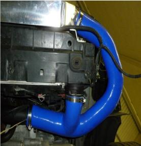
11. Place the bumper gently back onto the car, you may need to trim area shown below around the fog light bezel insert to help clear new intercooler. Also check the new silicon boost pipes are not pushing against the corner of the fog light carrier, if so trim corner as show in picture. Tip. On our demo car we remove some extra length off of the boost pipe where is connect to intercooler this help clear fog light carrier.
