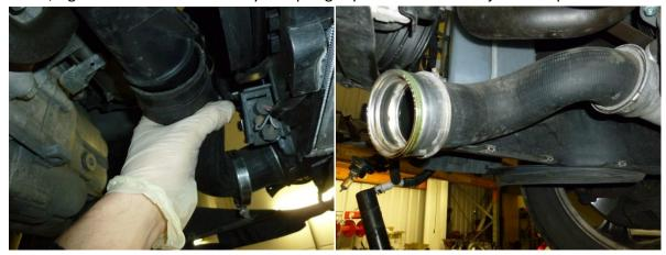
9. Remove seals from old hoses and install onto new billet alloy joiners, 2 x big joiners will go into standard Intercooler and small joiner goes to turbo pipe (closest to left hand side of sump pan) They will only fit in one way, once in re-install metal spring clips.
