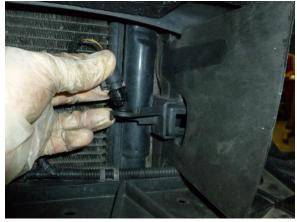
4. Remove left hand side horn bracket and install new Airtec horn bracket, this now locates on the headlamp lower securing bolt, remove bolt install bracket as shown below and secure, if headlamp washers fitted this may required adjustment when refitting bumper. Old horn bracket is used on Right hand side 'don't throw away'
