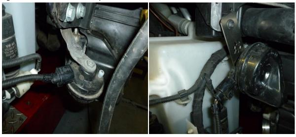
5. Remove Right hand side horn from bracket and remove old bracket, now take the Left bracket and fit as shown below, we have shown a finished picture to show why it has to be fitted this way. You will need to move Airflow wiring to the Right slightly so it reaches the mount on the intercooler as shown below.
