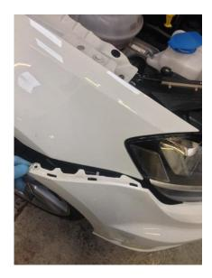
8. Remove bumper making sure to unclip multi plug and headlight washer pipe, unclip bonnet release sensor behind the bonnet release mechanism.
