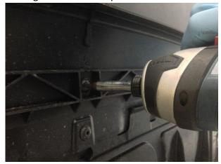
6. Undo 3x T30 Torx holding bumper to crash bar
