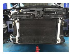
12. Unclip loom from plastic rad pack surround & unclip air con surround as shown.
