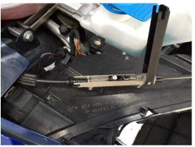
10. Remove crash bar 8x16mm bolts, 4x T27 Torx and horns. Make sure temp sensor is unplugged.
