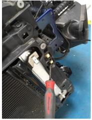
14. With a person's help remove the plastic rad pack surround - one person holding intercooler and radiator, the other removing the plastic rad surround.
