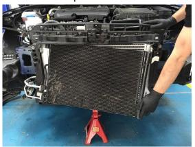
13. Use two flat blade screw drivers to unclip standard intercooler fixing clip securing intercooler to plastic rad pack surround (these will fracture/crack, please do not worry these will be firmly secured later using new fixings supplied).
