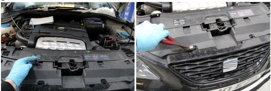
2. Remove x3 T25 from inner arch LH + RH side, also 1x T25 securing bumper to wing.
