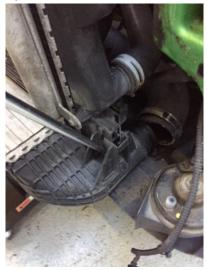
17.Install new intercooler, connect hoses & left and right brackets as shown.
