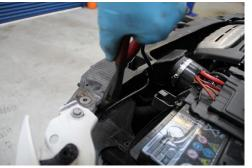
11. Remove wiring from left hand side of bonnet catch.
