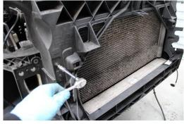
13.Remove the last x2 13mm bolts that secure the front rad pack.
