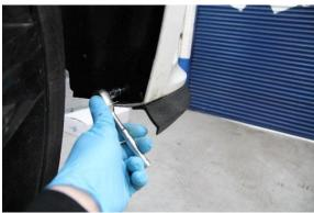
3. Remove 8x T25 screws securing bottom of bumper.
