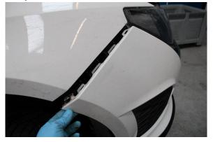
5. Remove bumper + unclip washer pipes if present.
