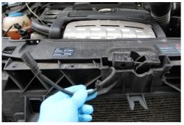
**12.**Remove T30 bolts securing rad pack onto the rad-pack support panel.
