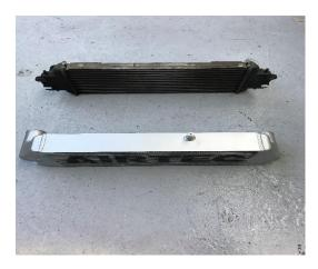
Fit your new Airtec intercooler by locating it in to the original lower pin locations. Then bolt the top of the intercooler in to place using the supplied m6x16 socket head and washer and Re fit boost pipes.
