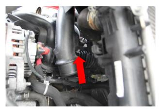
18. Install silicon & alloy boost pipes as per layout, right hand side is very tight due to not originally having boost pipe.
