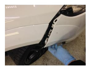
5. Remove bumper carefully and unclip loom multi-plug and block off washer pump with silicon pipe provided
