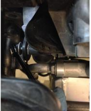
10. Install the intercooler by fitting the N/S first. Clip boost pipes on and secure with fittings provided onto OEM mounting points as shown in photo below:
