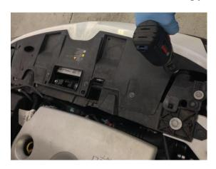
2. Remove 2 x T20 screws from inner wheel arch liner, also remove the x 5 plastic clips to enable more room to remove bumper
