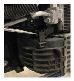
9. Un-clip intercooler pipes + remove cooler. Tip, remove 10mm bolt located @ top of drivers side boost pipe
